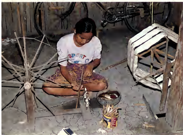
Young woman twists three filaments of silk (right) to make a single strand of 3-ply yarn (on the bobbin in front of her). Other bobbins of silk yarn are soaking in the bowl. Camba-camba village, 1986.
