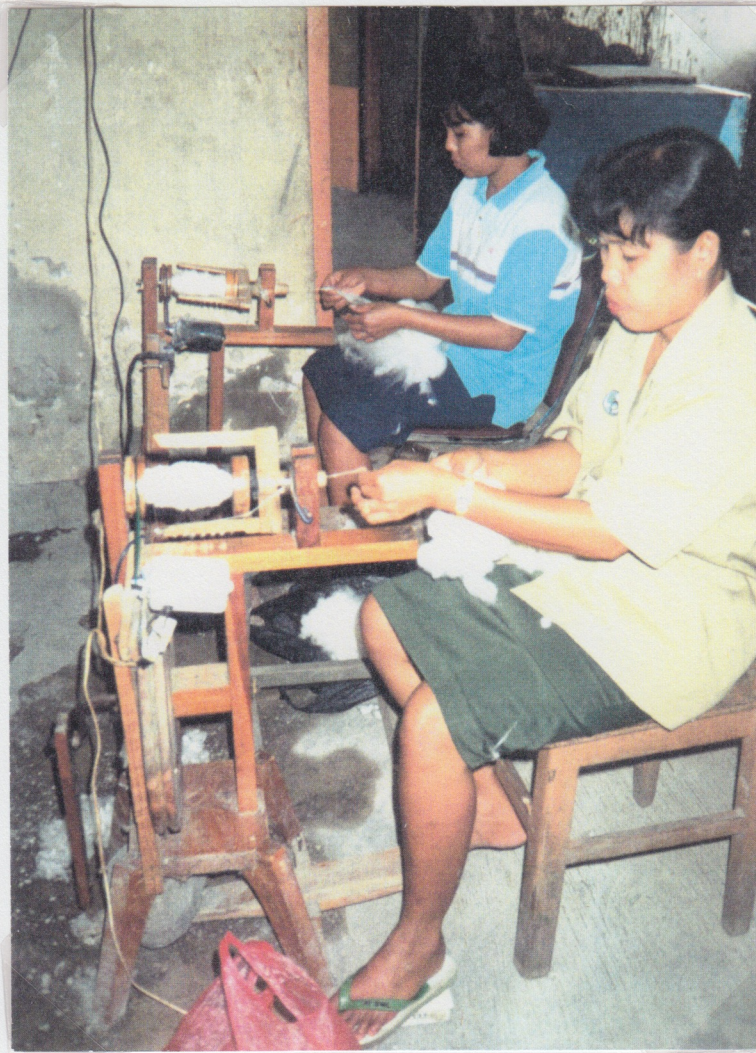
FIGURE 18 Cocoons that are cut (in order to remove the larva for breeding) no longer have a continuous silk filament. This silk has to be teased and spun like wool.
