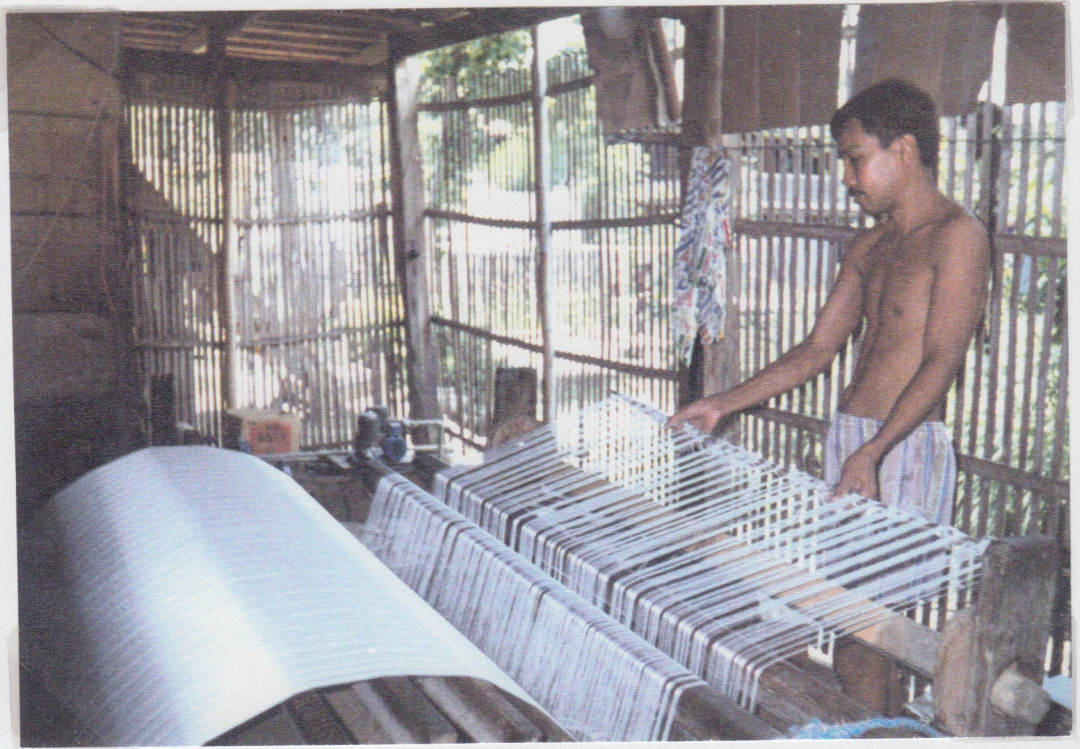
FIGURE 21 Warping-Up. Approximately 3600 warp threads will produce a one metre width of cloth. The second bar from the right will have 100m or 150m of thread wound on to it. Then it will be placed at the back of the loom with the threads running forward for weaving.
