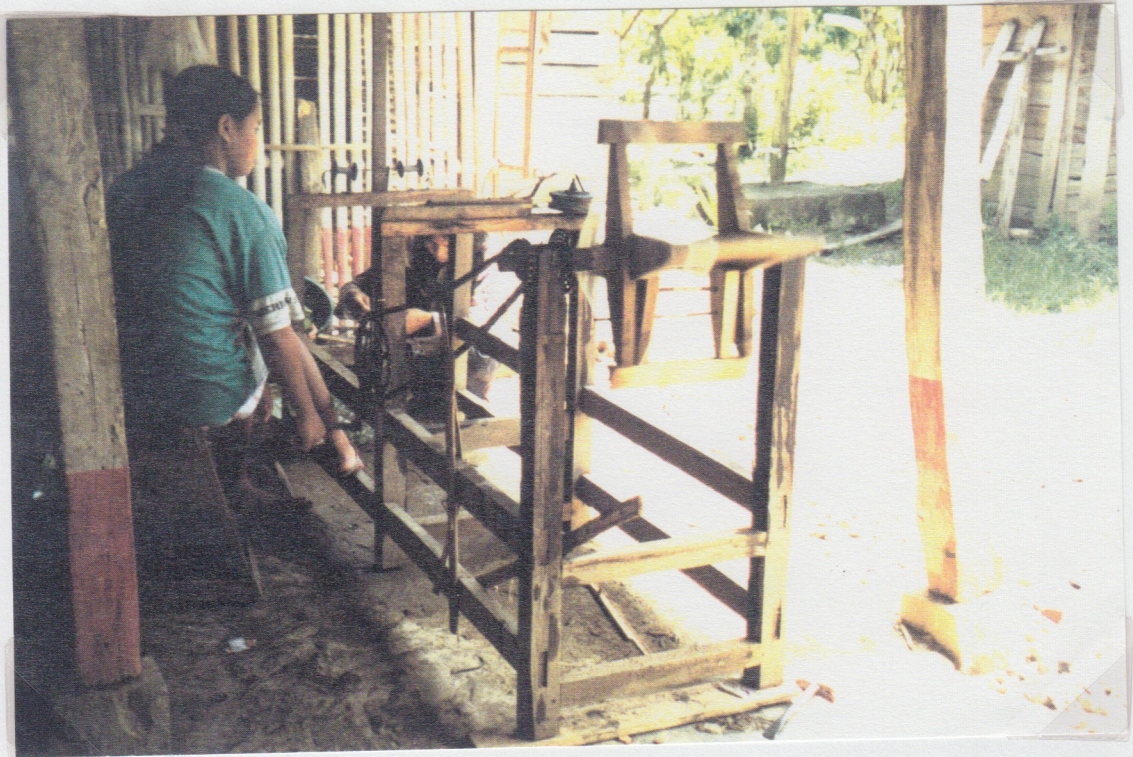
FIGURE 16 Silk thread can be reeled at home. Each filament can be up to 900m long. After reeling the neat hanks are dried and ready to be sold at the local market.
