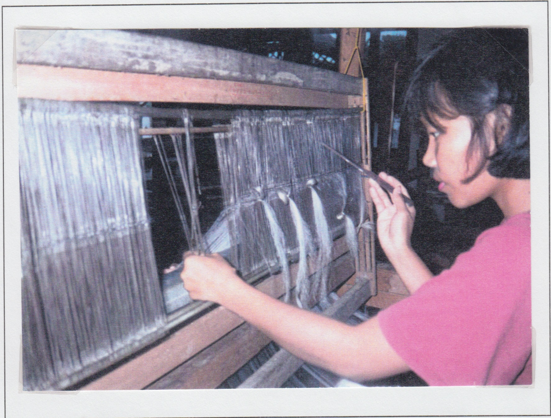
FIGURE 23 Threading up the loom. A two day process which includes separating the odd and even warp threads before weaving can begin.
